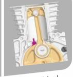
Reduced friction and constant ideal engine temperature by piston cooling jet, offset cylinder, and rocker roller arm working together.
